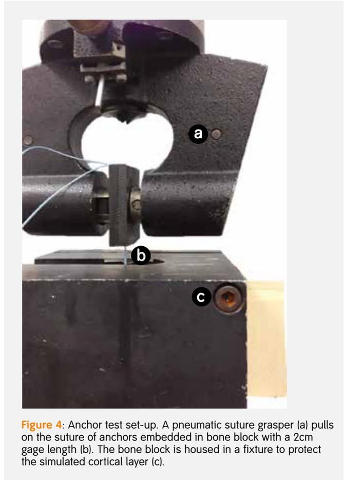
**Figure 4:** Anchor test set-up. A pneumatic suture grasper (a) pulls on the suture of anchors embedded in bone block with a 2cm gage length (b). The bone block is housed in a fixture to protect the simulated cortical layer (c).
