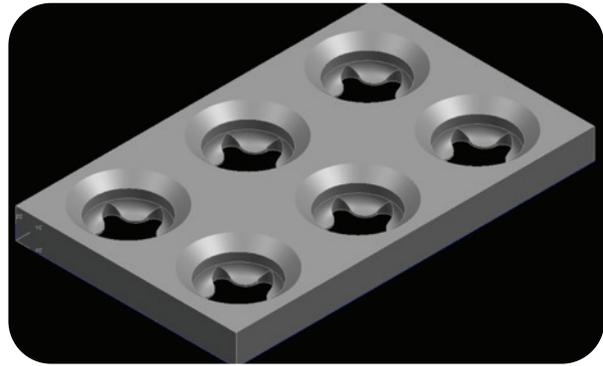
**Figure 2:** The test coupon used to simulate the locking tab features in the REDAPT Revision Acetabular System.
