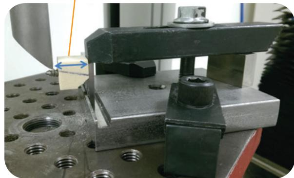
**Figure 3:** Static cantilever bending test setup. The test coupon is held in place and a load is applied to the end of the screw via the loading bar.
