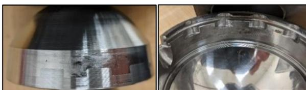
Fig. 3: Discoloration and fretting on the liner (left) and shell (right) taper surfaces of a CoCrMo construct after fatigue testing.
