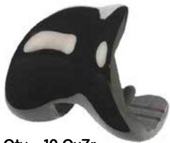
Qty – 10 OxZr Retrieved femoral components
