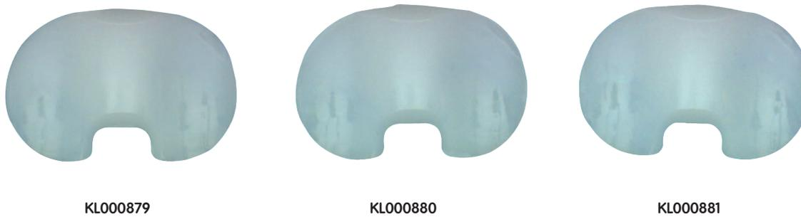
Figure 1: Wear patterns of XLPE tibial inserts after simulating 30 years of use.
